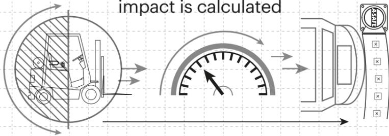
$\frac{1}{2} \text{ Mass} \times \text{Speed}^2 = \text{Joules}$
