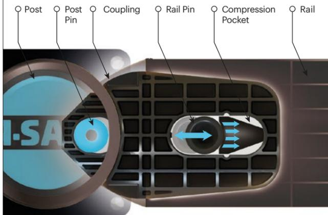
**PHASE 1:** Memaplex™ rail flexes to absorb impact, initiating the rail pin to slide forward and transfer load energy to the compression pocket.
