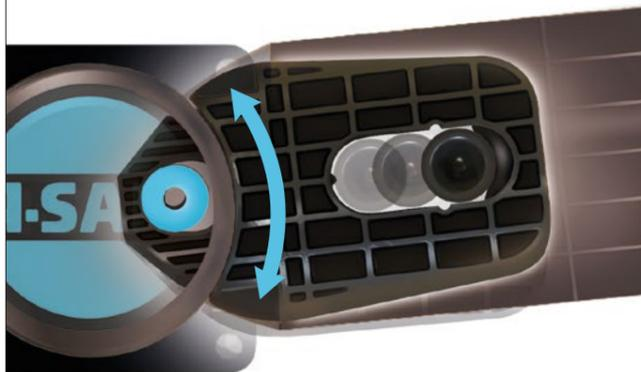
**PHASE 2:** Compression of the pocket continues to disperse energy as the coupling rotates around the post pin to activate further absorption.
